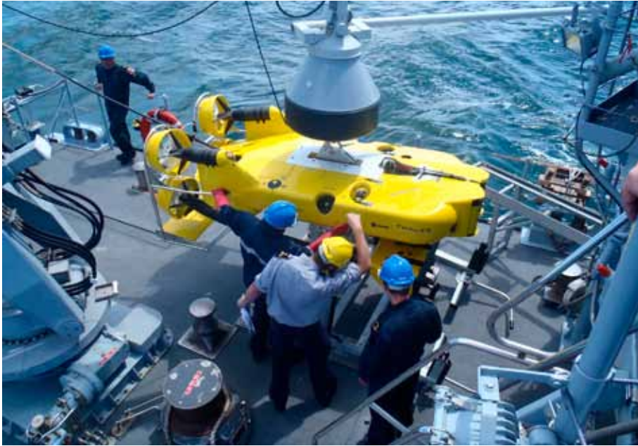
Self Propelled Variable Depth Sonar (SPVDS)
